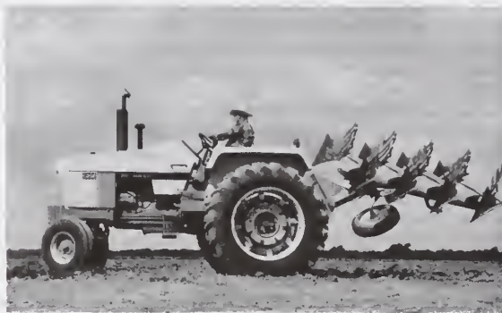
Figure 8: Tractor equipped with integrally mounted four-bottom two-way slat plow.
